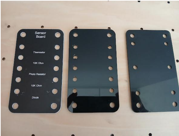
Figure 3: Left: Laser Cut Dual Layer ABS Plastic Five-Component Board overlay with component labels. Center: Laser Cut Acrylic Five-Component Board. Right: Laser Cut Acrylic, Three-Component Board.
