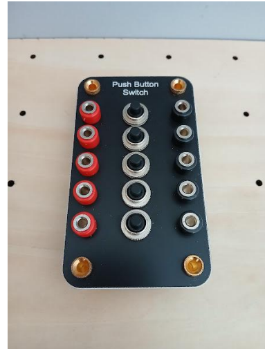
Figure 7 2"x4" Push Button Switch Board with Black and Red Banana Connectors
