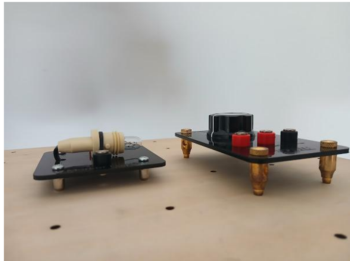
Figure 4 Left: 2"x2" Marker Lamp Bulb with Pomona Electronics Standoff. Right: 2"x4" Potentiometer board with Flutesan Standoff.
